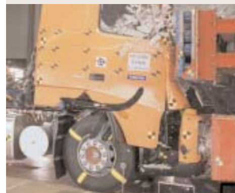
Single accidents involving trucks are simulated using the Swedish cab strength test – the toughest and most realistic safety test in the world. Collisions between two trucks are simulated by means of Volvo's unique barrier test.
