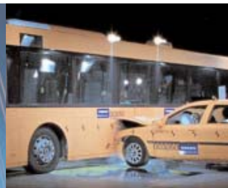
Volvo Buses also carries out full-scale collision testing to assure the safety of passengers in low-floor buses. The test shown here is between a car and a city bus.
