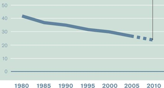
Development of fuel consumption, Volvo truck model FH12, 40 tons.
