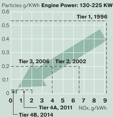
Nitrogen oxide and particulate emissions have fallen by about 60% since 1996. When Tier 3 was introduced, Volvo Construction Equipment launched products equipped with the new V-ACT technology (Volvo Advanced Combustion Technology), which minimizes emissions by adjusting the combustion process in the engine. Nitrogen oxide and particulate emissions will decline by a further 90% by 2014 compared with today's Tier 3 level.
