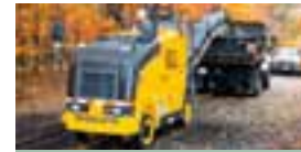
Asphalt milling machines
