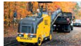
Asphalt milling machines
