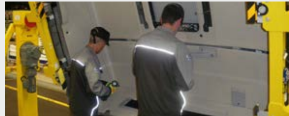
Ergonomic improvements on assembly lines for new Renault trucks have transformed 50% of workstations that previously had an average 'high' and 'heavy' ergonomic quotation to the lowest level.
