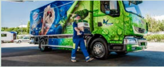
Fully electric trucks emit no particulate matter, nitrogen oxides or carbon dioxide during operation and have very low noise levels, making them suitable for city distribution.
