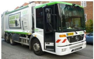
• Most effective measure: Lowered cabin and glass door "In all of the accidents that were analyzed, the truck driver would have had at possibility to see the cyclist, if the driver had used the right mirrors at the right time and taken the nessesary time to orientate"
