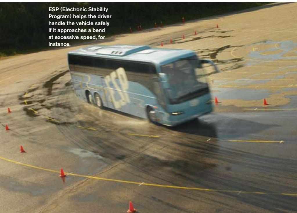
ESP (Electronic Stability Program) helps the driver handle the vehicle safely if it approaches a bend at excessive speed, for instance.
