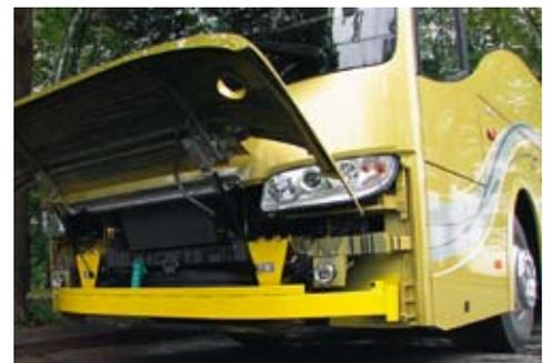
FUPS – front underrun protection to reduce the consequences on a car of a collision with a coach.
