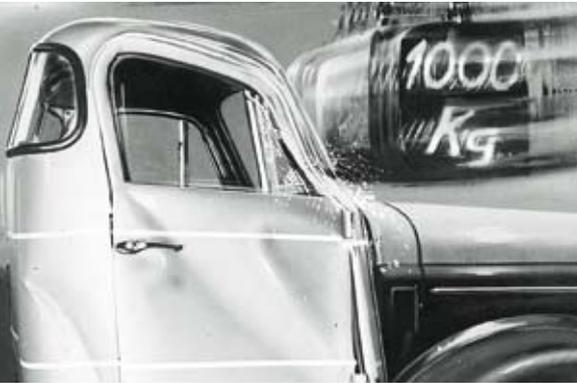
The Volvo Group's impact test for truck cabs was introduced in 1960, before legislation required such tests.
