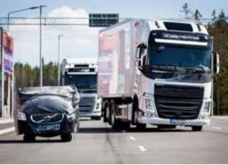
In order to further develop active safety systems, complex traffic scenarios are created on the test track.
