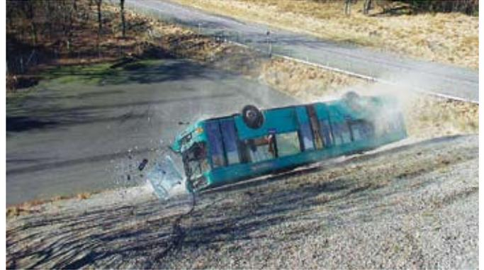
Full-scale collision tests are carried out, for instance rollover tests with buses.
