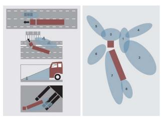
Figure 4. Truck seen from above. The numbered fields, 1–8, show areas that can be difficult for the driver to see.
