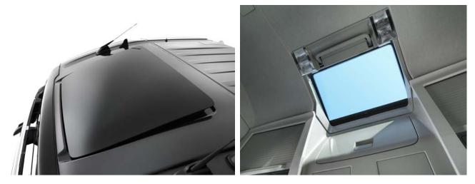
Figure 7: The roof hatch in the new FH functions as escape path in case of a vehicle roll over accident.
