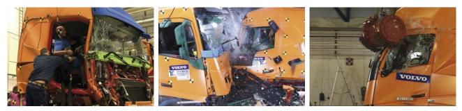
Figure 2: An illustration showing the knowledge gained from crash tests (crash facility testing, full scale test of new FH, pendulum testing) and a picture showing the investigation of an accident in the field.
