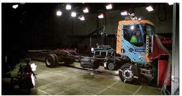
Physical full-scale impact tests supplement the development engineers' collision simulations.
