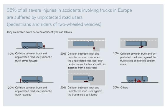
The Volvo Trucks Accident Investigation Team maintains a massive database of parameters such as accident types and the kinds of injuries suffered in accidents. In recent years, special attention has been paid to studying the relationship between trucks and unprotected road-users.
