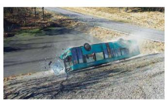
Full-scale collision tests are carried out, for instance rollover tests with buses.
