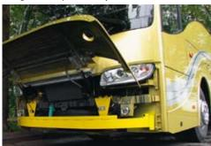
FUPS - front underrun protection to reduce the consequences on a car of a collision with a coach.
